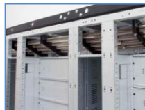
Rear Bar Cabinet: segregated compartment cabinet in form 3b. Vertical busbar system positioned in the rear area and horizontal busbar system positioned in the upper area.
